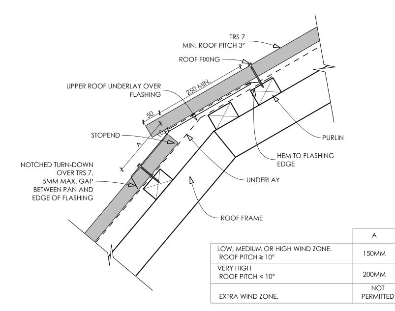
These details are generally in accordance with E2/AS1 and or the NZ metal roof & wall caldding code of practice.
