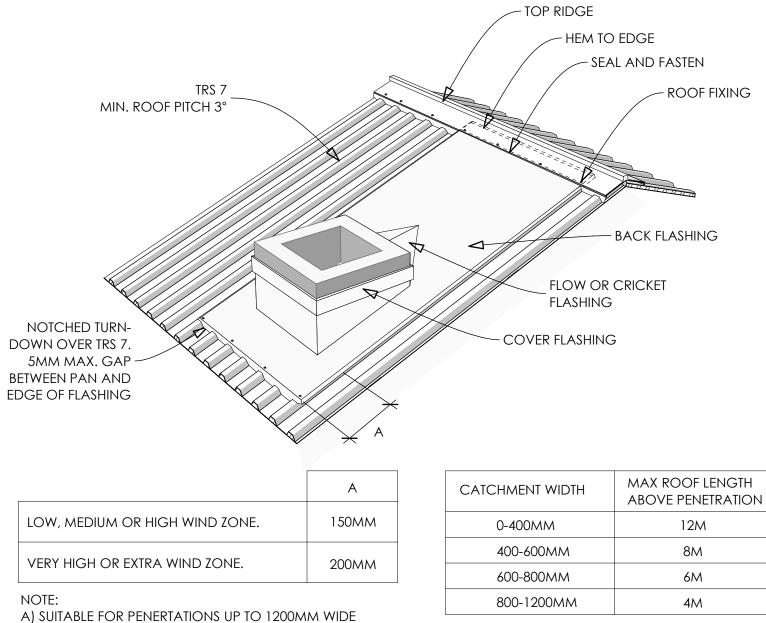
These details are generally in accordance with E2/AS1 and or the NZ metal roof & wall caldding code of practice.
